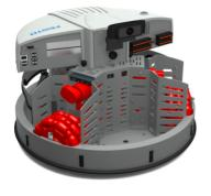
The wheel technology to do this has existed for some time and is regularly used in education, hobby and toy robotics in two forms. One is commonly referred to as an Omni-wheel, and the other a Mecanum wheel. Although somewhat different, they both use rollers on the outer perimeter of the wheel to allow movement in any direction. Essentially they have wheels within a wheel, and can be used to drive the robot in any direction.
