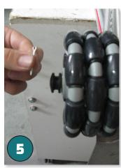
Align the holes in the axle cap with the holes in the axle.
