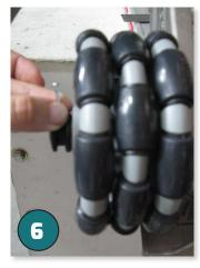
Insert 1 x split pin through the holes in the cap and the hole in the axle.
