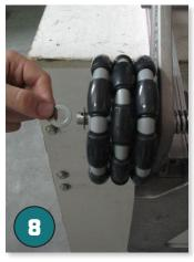
If it moves more than 2mm, remove the split pin and axle cap and insert another thin washer between wheel and axle cap.
