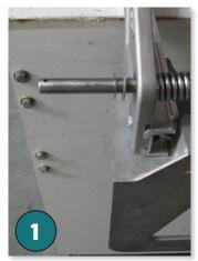
Place Rotatruck on a bench to have access to the wheel base. Then slide 1 x thick and 1 x thin washer onto the front stub axle.
