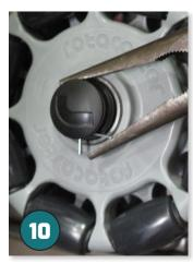
Bend the split pin legs apart and around the axle cap.
