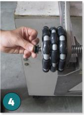
Place axle cap on the end of the stub axle.
