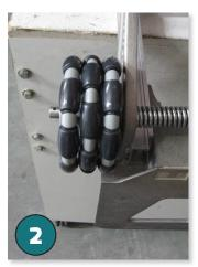
Slide the Rotacaster Wheel onto the front stub axle.
