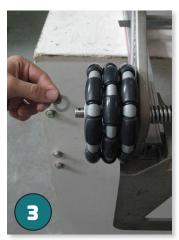
Slide 1 x thin washer on the front stub axle.
