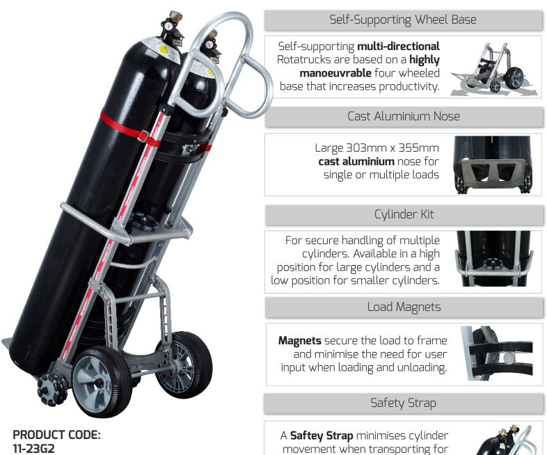
Load Capacity: 230kg Dimensions: 1700 x 500 x 600mm
