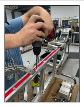
Step 2: Drill out the hole which is 6.5 mm to 8.5 mm using a 8.5mm drill bit.
